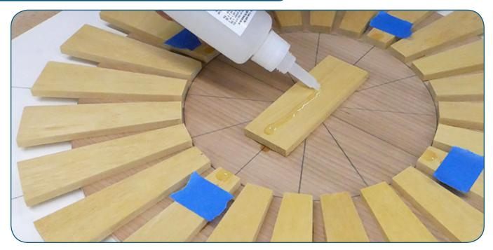
Glue the Filler Block over the center of the Back. Then center the Face on the Petals and apply painter's tape to mark the edges of the Face. Apply a bead of glue to the Filler Block and next to each piece of tape.
