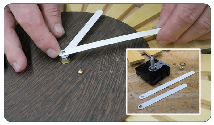
Drill a 5/16" hole through the center of the clock face. Follow the installation instructions for the clock mechanism.
