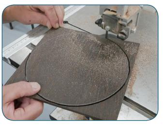
Use a compass to draw the 13"-diameter perimeter on the Back piece (left). Then cut the wenge Face (A) stock into 8"-long pieces and edge glue them together to make the Face piece. Next, mark a 7-7/8" circle in the center of the Face piece. Cut out both pieces (right). Cut just outside the line on each piece and sand flush to the line.
