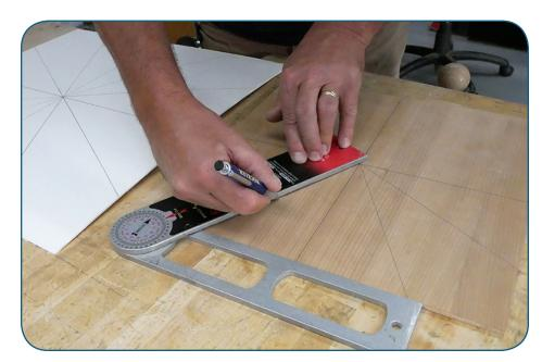
Refer to the Petal Layout Detail drawing on p.3 and use a protractor or angle-finder tool to mark the petal alignment lines on the cherry plywood Back (C) and on a piece of paper that is at least 16" x 16". The paper will be used to help align the petals.
