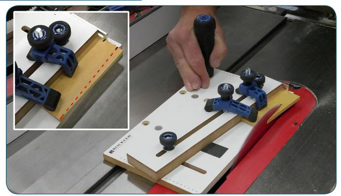
Cut twenty-four petal pieces to 1-3/8" x 4-1/4". Each petal will taper from 1-3/8" wide to 5/8" wide (see Petal Detail, p.3). Use the Small Parts Taper Jig (57550) and table saw cut the tapers along both long edges of each petal. Set up the first taper cut to follow a line from the front corner to a mark that is 3/8" in from the opposite corner (inset photo). Make this first taper cut on all twenty-four petals.
