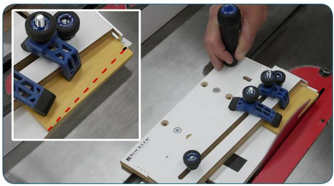
Next, flip each petal over to taper cut the same taper along the opposite edge. You must reset the Small Parts Taper Jig to cut a line from the front corner to a mark 3/8" in from the opposite corner (inset photo).
