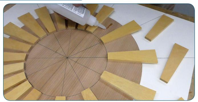
Use a compass to draw a 3-1/2" radius circle on the Back. Place the Back on top of the paper and align the layout lines on the paper and the Back. Attach a petal over each layout line with glue. Apply a bead of glue on the line and center the petal over the layout line with the narrow end tangent with the inside circle. Use the lines on the paper to help align the wider end of each petal. Next, attach a petal between the petals that have already been attached.
